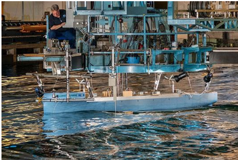
Figure 4.3. wPCC tested at RISE SSPA Maritime center. Copyright 2020 by RISE.
