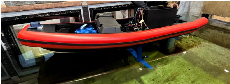
Figure 45 - SSRS06 foiling model boat designed for Swedish Sea Rescue Society and manufactured by Aston Harald.
