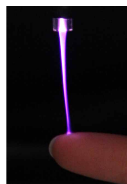
Figure 1. Typical demonstration of non-thermal plasma.
